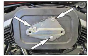
3. Remove the three bolts securing the factory air filter and bonnet bracket and the remove the factory air filter.
