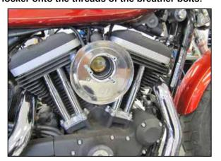
8. Install the filter back plate and secure with the filter spacer bolts.
